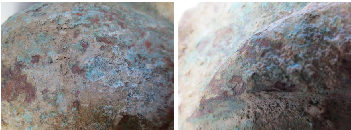
Weathering layers of low tin bronze, incrustated with soil particles.
