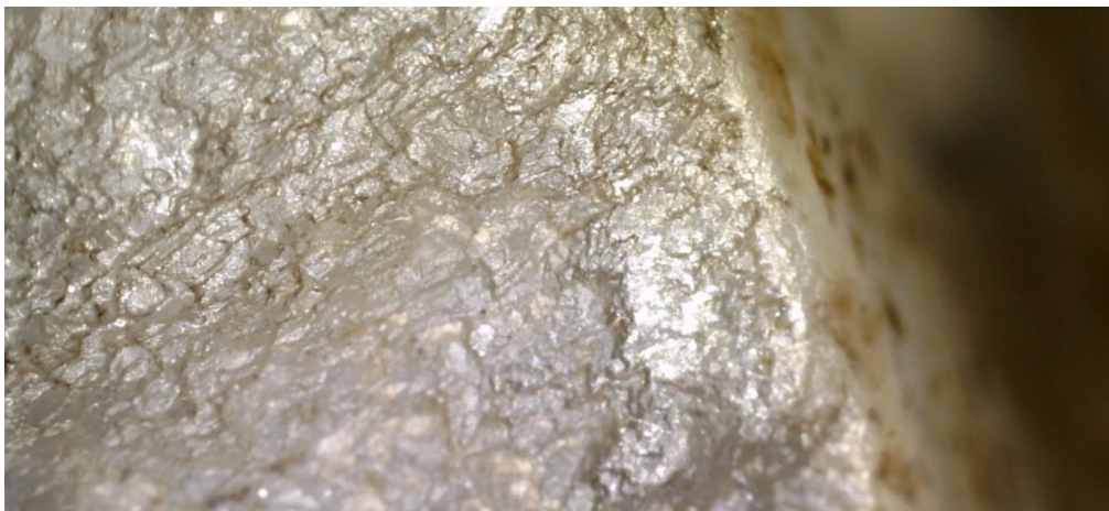
Detail (x200, polarized light): the fracture plane on the left ear is recent ( \leq 200 years).
