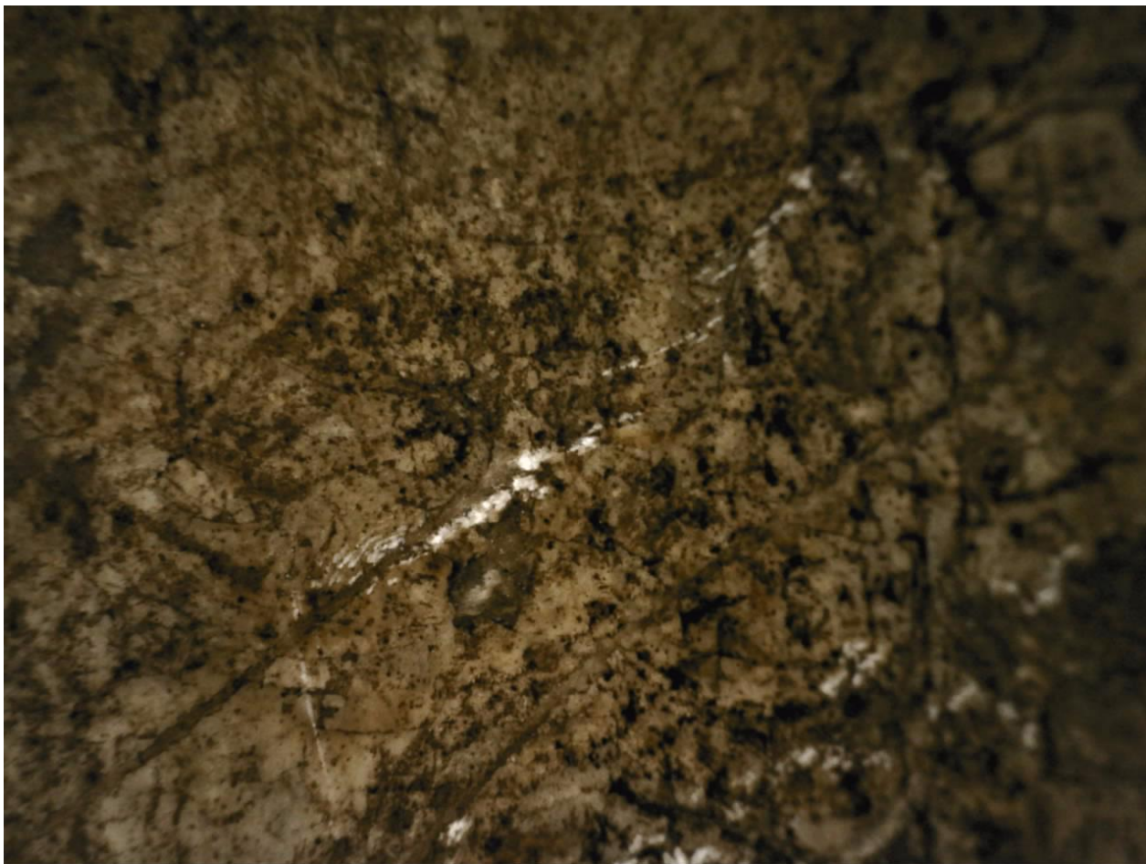
Surface structure detail (x150, incident light): handmade random polishing marks.
