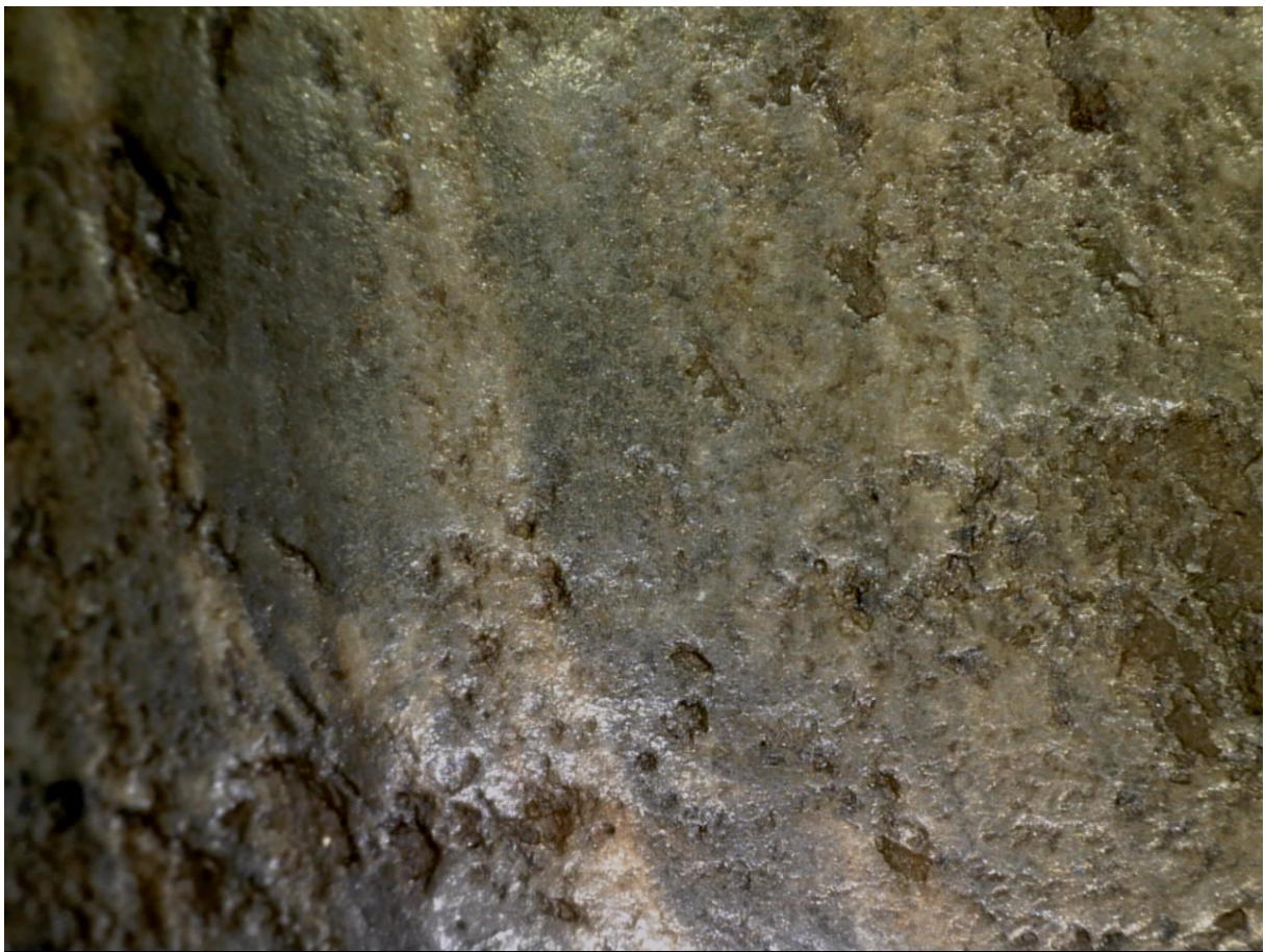
Quartz area at the right side of the mask with the less weathered surface. (x50, incident light)
